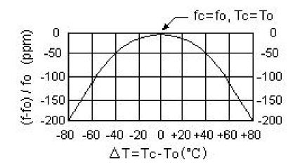
The curve shown above accounts for resonator contribution only and does not include LC component temperature contributions.
